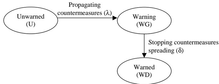
Fig. 2. The state machine of spreading countermeasures
