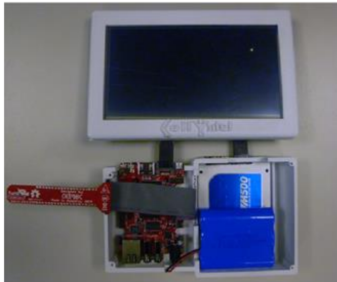
Figure 3. CellIntel prototype's components during the manual assembly: LCD screen, 3D printed screen case, battery, SSD hard disk drive, printed circuit board, cables for connections among components and 3D printed base case.
